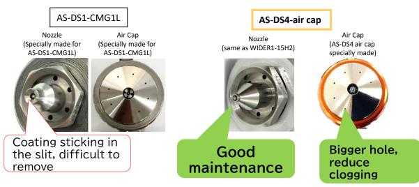
Disadvantage of AS-DS1-CMG1L is the difficulty of nozzle cleaning, while for AS-DS4, it uses the same nozzle as WIDER1-15H2S(G) and nozzle cleaning becomes easy.
