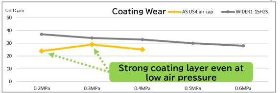
[Application Condition] Coating: GENJYU HLP-8181 / Dilution: Coating 1 to Water 1 (by weight ratio) / Application Starting Temp.: 230°C / Distance: 200mm
