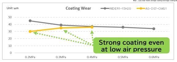
%Application Condition→Coating:GENJYU HLP-8195/Dilution Ratio:Coating 1 to Water 1 (weight ratio)/Application Starting Temp.:230°C/Distance:200mm/Discharge Volume:Open 2/4 from completely closed condition
