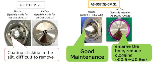
Disadvantage of AS-DS1-CMG1L is the difficulty of nozzle cleaning, while for AS-DS7(G)-CMG1, it uses commonly-used straight nozzle (nozzle diameter 1.0) and improves nozzle cleaning.
