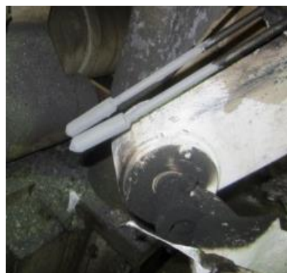
After use: No aluminum attachment (after 2 shifts operation) No need for maintenance for 1 week
