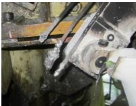
Before use: Aluminum oxide attached ADC12, 680°C
